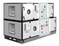
The advantage of Econet is that it combines all energy functions, recovery, heating and cooling are integrated into one package. Combined with Aquacool recovery system the resultant increased efficiency in heat transfer means far lower hot water temperatures (40/30°C) and far higher chilled water temperatures (14/18°C) can be utilised.
